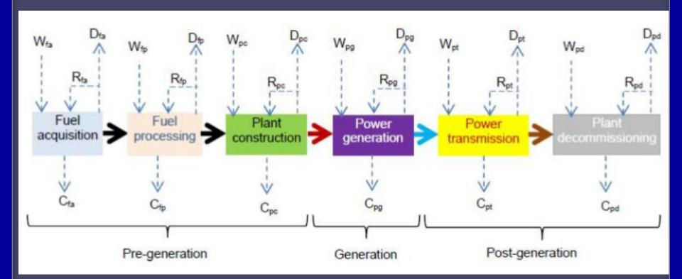
Framework for water use analysis in the energy production. C=consumption, D=discharge, R=recycled, W=withdrawal.
